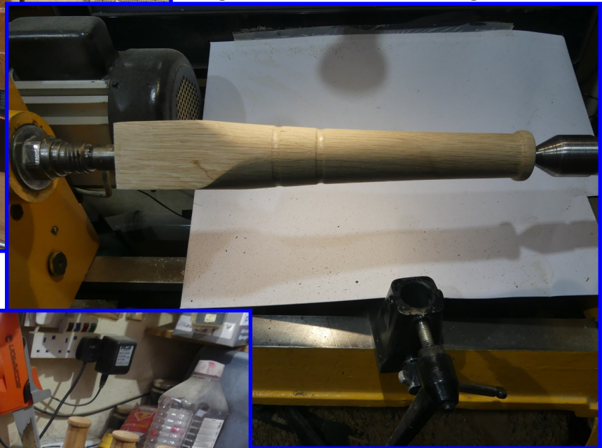
The light bodies are turned into their final shape.
